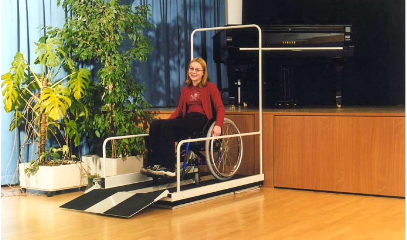
A bellow covers the LIFTboy on all four sides and provides protection from contusions. An additional fixed banister serves as protection of the upper landing. The long sides are equipped with a safety edge and a 40 cm high banister.
